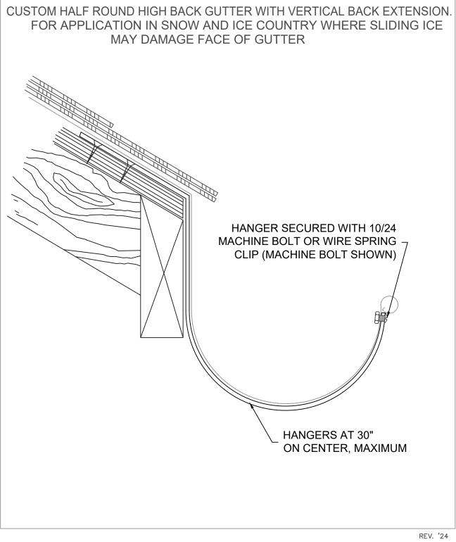
IN AREAS SUBJECT TO SNOW SLIDE, COORDINATE THE FRONT EDGE ELEVATION OF GUTTERS WITH ROOF SLOPE LINE.
