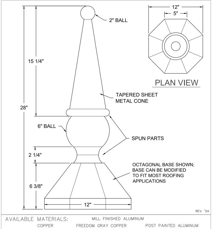
WEIGHT: VARIES DEPENDING ON ROOF CONDITION, ROOF SLOPE AND MATERIAL INSTALLATION: SEAL THE MOUNTING BRACKET (PROVIDED) TO THE ROOF SURFACE FOR
