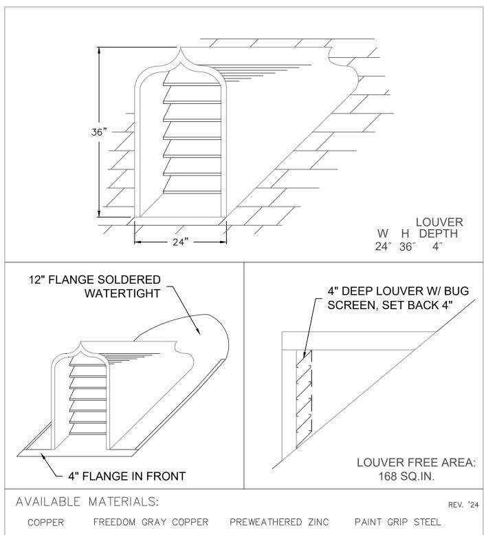
INSTALLATION: MARK OPENING IN ROOF DECK ON DESIRED COURSE. CUT OPENING IN DECK. POSITION DORMER OVER OPENING AND FASTEN TO DECK.
