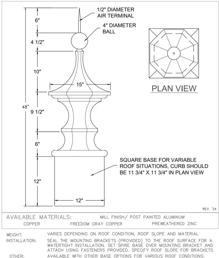
OPTIONS: AVAILABLE WITH LIGHTNING PROTECTION KIT. CONTINUE L.P. SYSTEM AS PER LOCAL CODE BY QUALIFIED LIGHTNING PROTECTION INSTALLERS.
