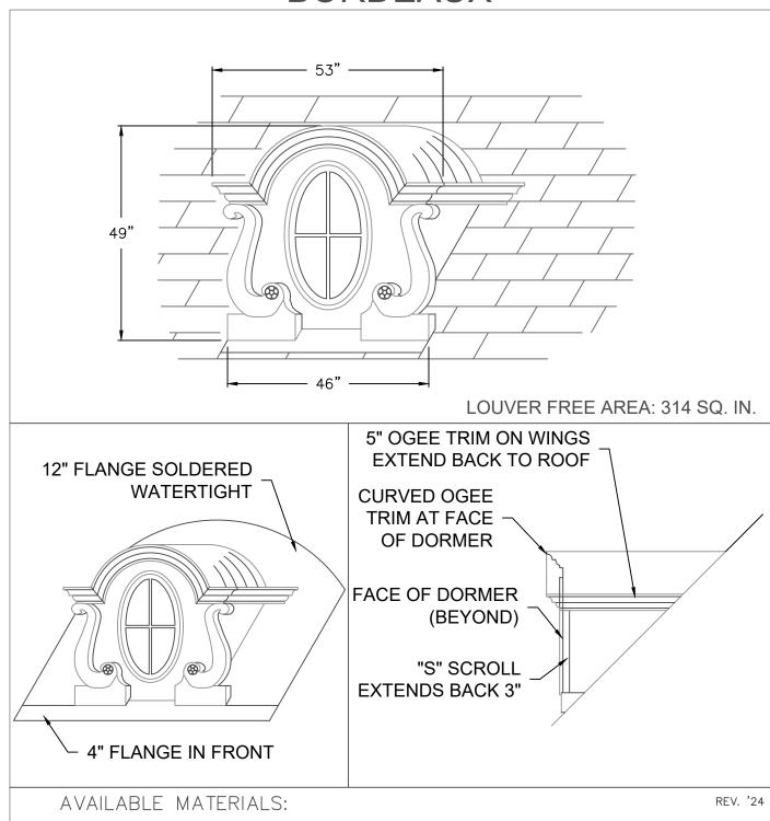
INSTALLATION: MARK OPENING IN ROOF DECK ON DESIRED COURSE. CUT OPENING IN DECK. POSITION DORMER OVER OPENING AND FASTEN TO DECK.
