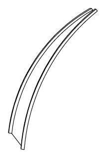
CURVED AND TAPERED PANELS FOR DOME ROOFS
