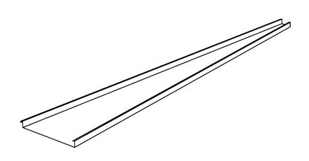
STRAIGHT TAPERED PANELS FOR CONE SHAPED OR TURRET ROOFS
