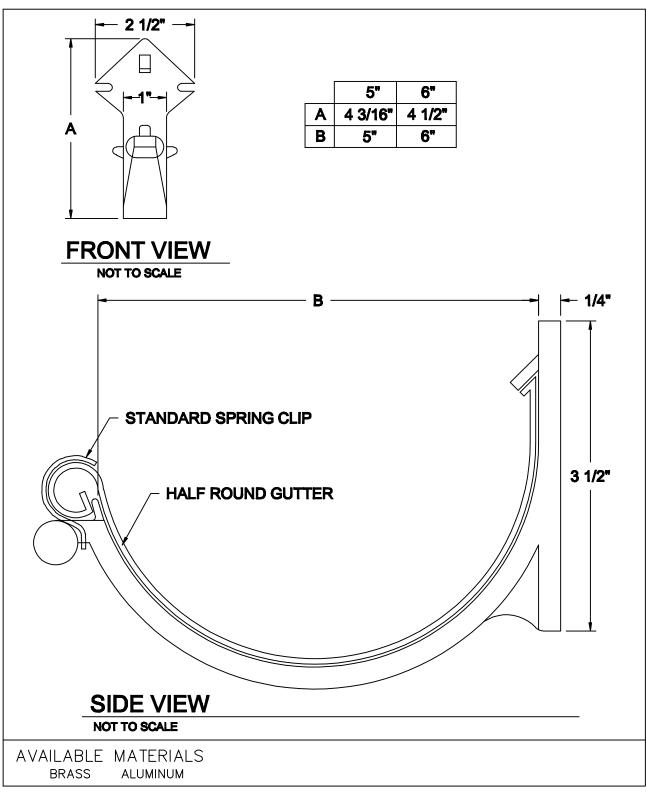
IN AREAS SUBJECT TO SNOW SLIDE, COORDINATE THE FRONT EDGE ELEVATION OF GUTTERS WITH ROOF SLOPE LINE. REV. 7/14
